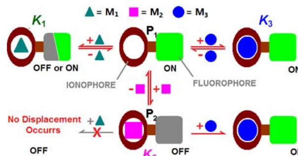
Figure 1. Illustration of the transformation from a nonselective fluorogenic receptor ( P_1 ) to a selective OFF–ON FCS ( P_2 ) for metal cations through quencher displacement. K_1 , K_2 , and K_3 represent the binding constants for the interference ( M_1 ), quencher ( M_2 ), and target ( M_3 ) metal cations, respectively; K_1 < K_2 < K_3 .
